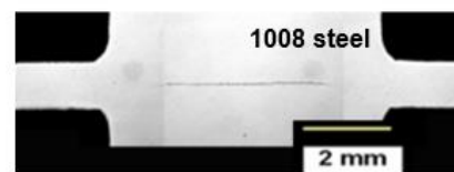
Fig. 8 Elongated cracks along a localized ASB in (a) 1038 steel (aspect ratio= 1.8, drop height= 2.4 m, drop weight= 30.5 kg) (etchant: 2% Nital solution) (b) 1008 steel (aspect ratio= 1.6, drop height= 2.4 m, drop weight= 37.6 kg)
